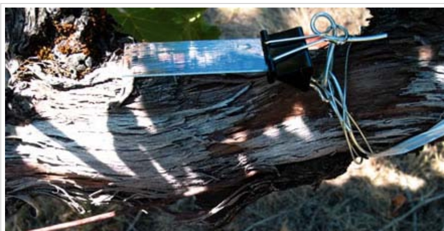
A spore trap (above) is useful to vineyard managers looking to pinpoint which fungi are present.
